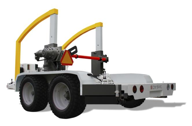
Soundly constructed drum carriers for slowtraffic. With an impressive range of user advantages. With or without drum drive. For load carrying weights from 11 up to 30 tonnes.
